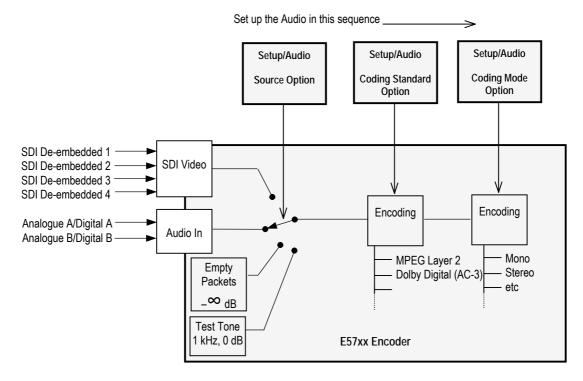
Figure 4.14: Setting up the Audio Input
